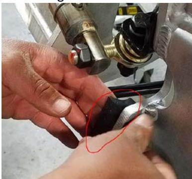
11. Lower the breakaway and check alignment of dampers by looking down the end of the breakaway and verifying they are in line with the secondary bottom rails (see below).
