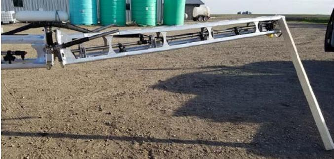
4. Using 7/16" wrench and 5/32" allen wrench remove poly blocks, both sides. Place poly bushings on bolts for reinstallation.
