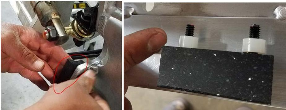
5. Lower breakaway back down after Poly blocks are removed. This is necessary as the dampers have an 1/8" of preload and will not be able to be removed without removing the tension.
